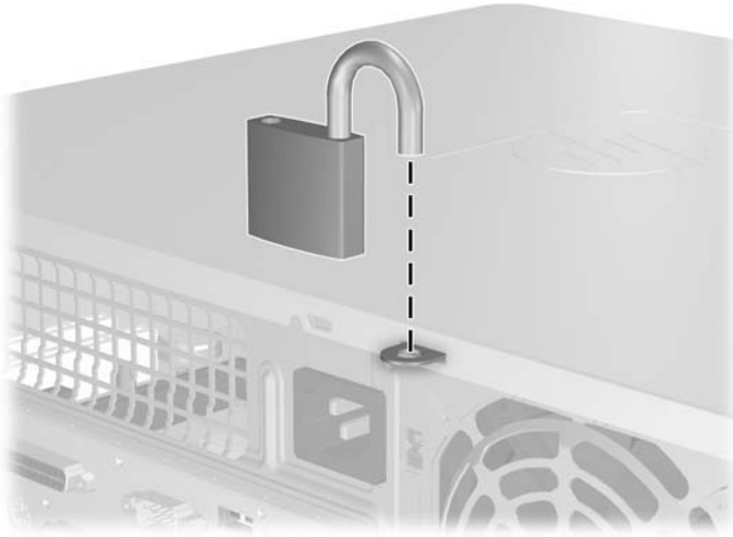
Figure C-2 Installing a Padlock
