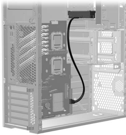
Figure 4-56 Connecting the data cable
