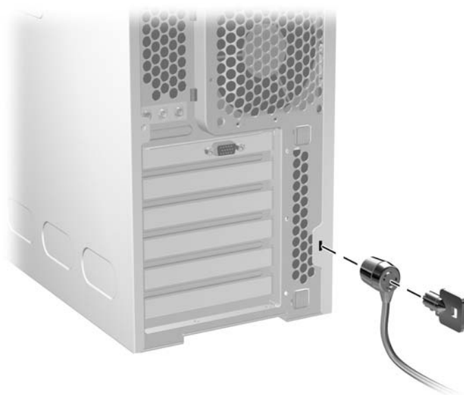
Figure 4-3 Removing the cable lock
