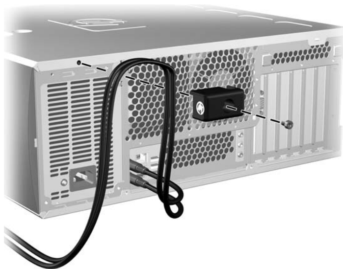
Figure 4-4 Unlocking the device
