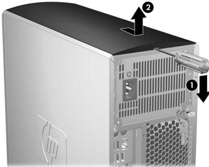
Figure 4-7 Removing the top cover
