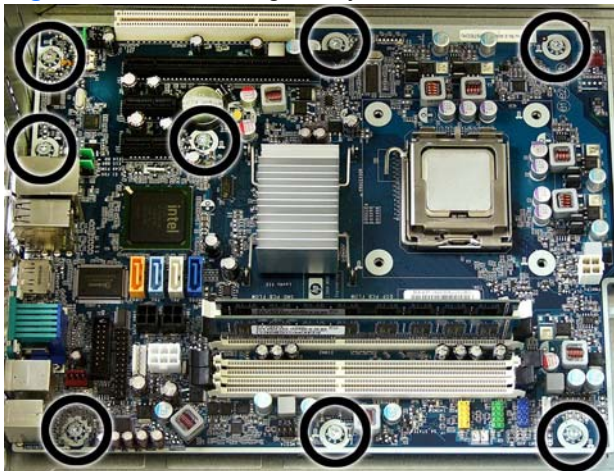
Figure 9-54 Removing the system board
