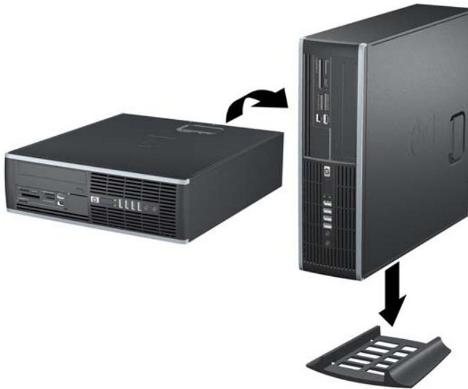
Figure 9-66 Changing from Desktop to Tower Orientation
