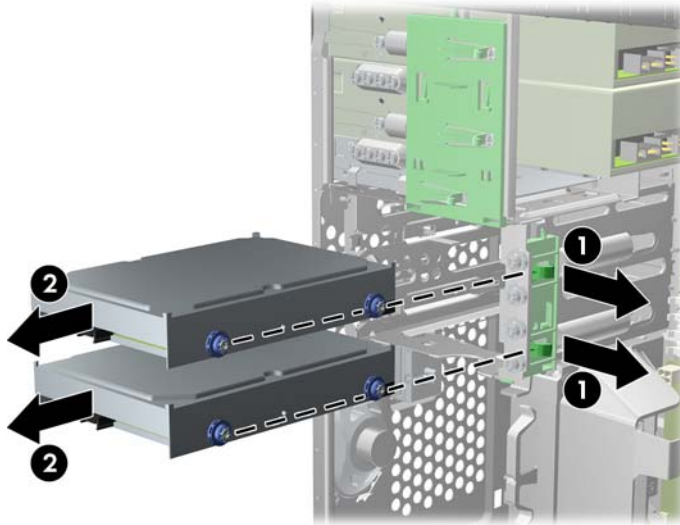
Figure 8-26 Removing a Hard Drive
