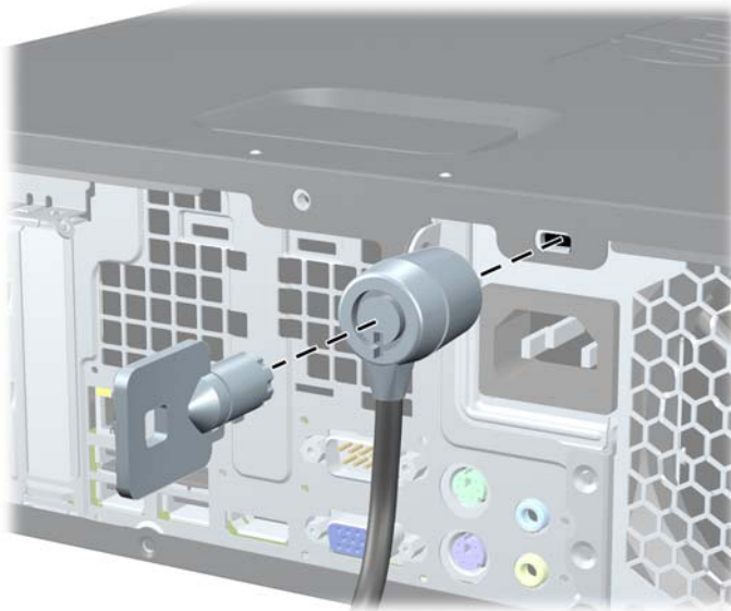
Figure 9-58 Installing a Cable Lock
