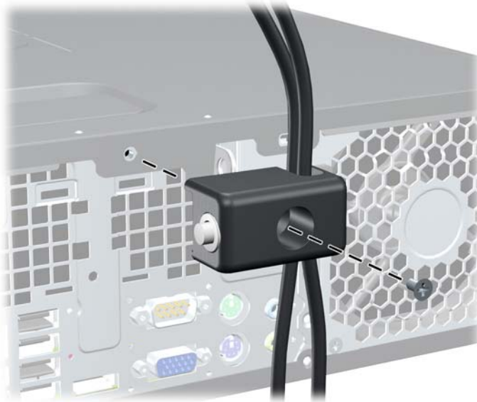
Figure 9-62 Attaching the Lock to the Chassis
