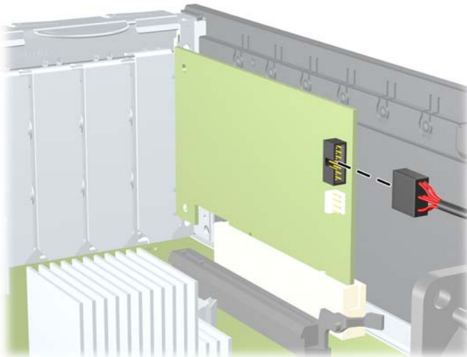
Figure 9-28 Disconnecting the Media Card Reader 1394 Cable
