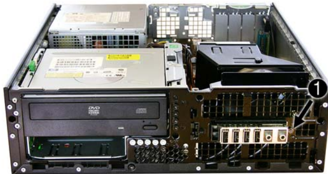
Figure 9-47 Removing the front I/O device/power switch
