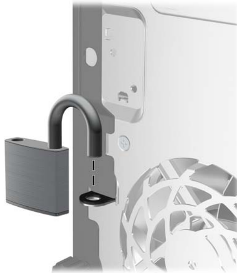
Figure 8-39 Installing a Padlock
