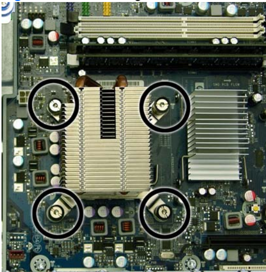
Figure 9-51 Removing the heat sink
