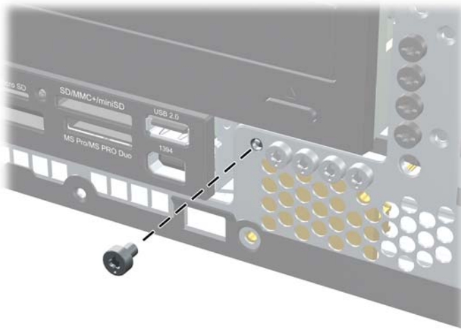
Figure 9-64 Retrieving the Front Bezel Security Screw
