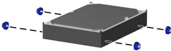
Figure 8-27 Installing Hard Drive Guide Screws
