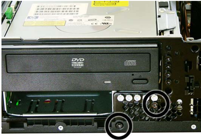
Figure 9-50 Removing the speaker
